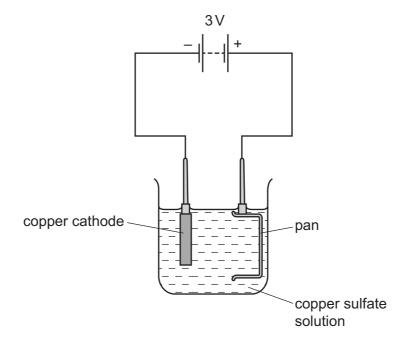
Which action will plate the pan with copper?
